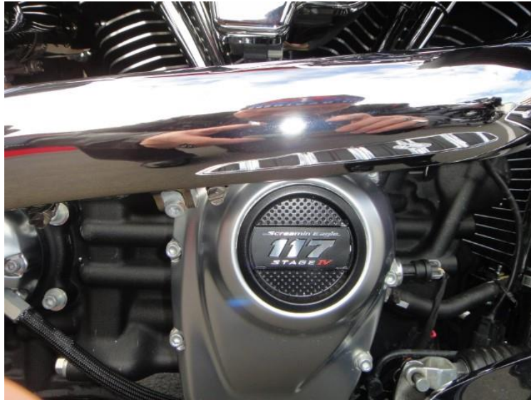
Image 12 - Not satisfied with the already impressive performance of his stock bike, Jimmy has opted for the Screaming Eagle upgrade kit taking his bike from 114 cubic inches to 117 cubic inches along with other performance enhancing bits and pieces.
