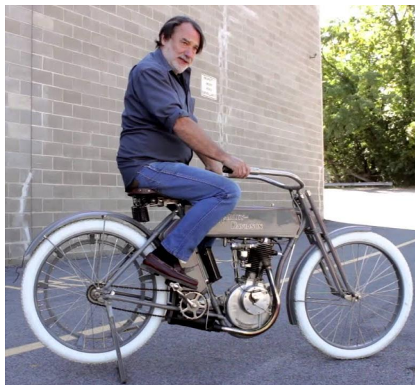
Image 27 (downloaded) - The first Harley-Davidson's differed little from other motorcycles of the time, essentially being a bicycle powered by a simple single-cylinder motor that drove the rear wheel through a leather belt. The normal pedals and chain remained in place so the rider could pedal the bike up to speed to start the motor, as well as lend a little leg power when ascending hills.
