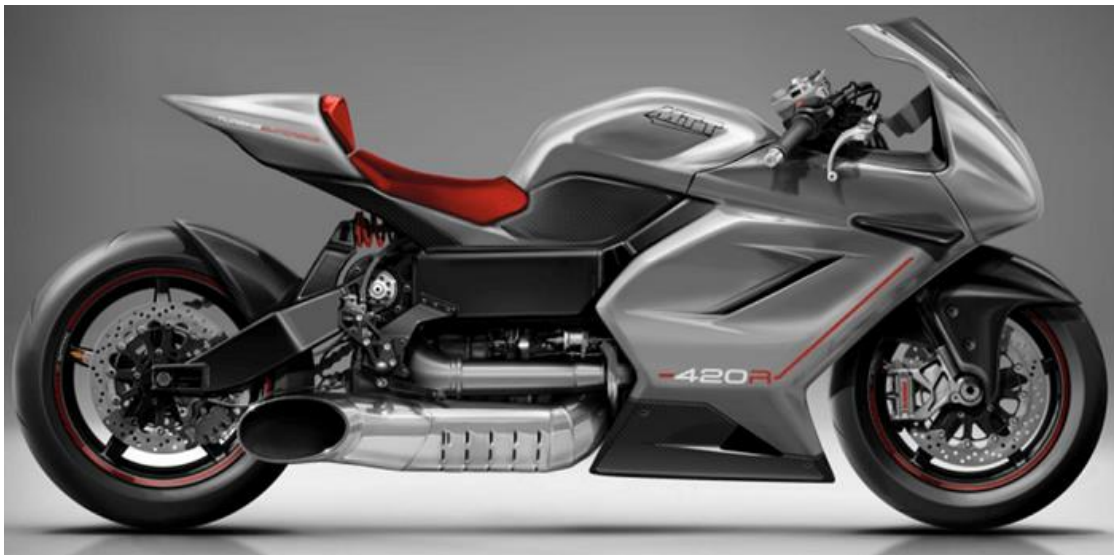
Image 55 (downloaded) - The MTT Turbine Superbike, which is powered by a Rolls Royce Allison turbine engine, cost $185,000 in 2004, making it the most expensive production motorcycle ever to go on sale. The bike's Rolls Royce turbine engine produces 213 kW (286 hp) of power at the rear wheel.
