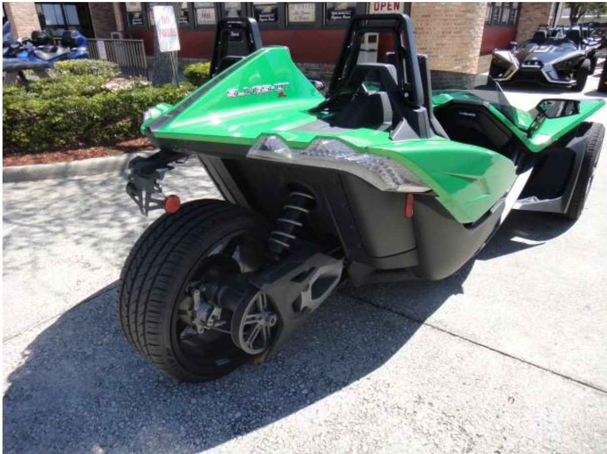
Image 37 – The rear of the Slingshot vehicle. This vehicle is driven by the back wheel; it has an in-line 4-cylinder 2.4 l motor, 5-speed manual gearbox, and has no roof, doors, or side windows, no airbags or crumple zone.
