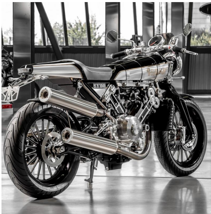
Image63 – Evoking the style of its Jazz-age forebear as well as being constructed out of the latest cutting edge components; this new motorcycle makes no compromises when it comes to quality and design. The new engine is a DOHC 8 valve, 880 water cooled V-Twin with a six speed gearbox and displacement of 997cc. The new SS100 is a highly sophisticated ultra-modern machine with a jazz age, Art Deco look but improved to beyond modern standards with exclusive technologies and the finest materials.
