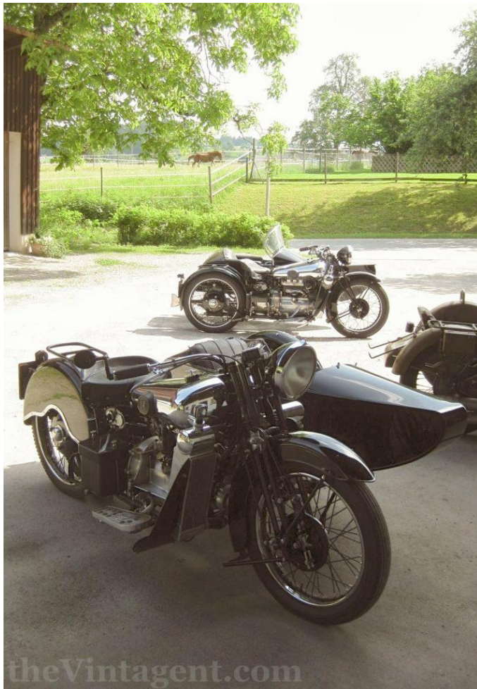
Image 41 – The BS4. Note the water cooled engine with radiators on each side of the engine. This had a 4-cylinder engine and transmission straight out of an Austin Seven motor car.
