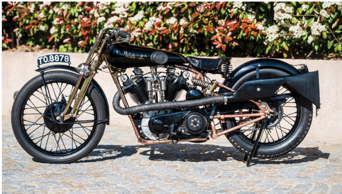
Image 22 - This 1928 Brough Superior SS100 nicknamed "Moby Dick" was a George Brough one-off special featuring a 1,140cc JAP engine, and with other engine performance modifications it was capable of 115 mph (185 km/hr) in 1928. It was specially tuned by George Brough and JAP. In 1931, Motor Cycling magazine described this bike as "the fastest privately owned machine in the world".
