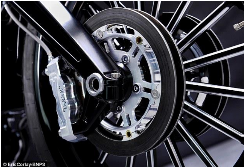
Image 65 - One interesting modern update is the incredibly powerful quad-disc brakes up front which have taken braking to a whole new level. The brakes are from Beringer and are sourced from the aircraft industry.
