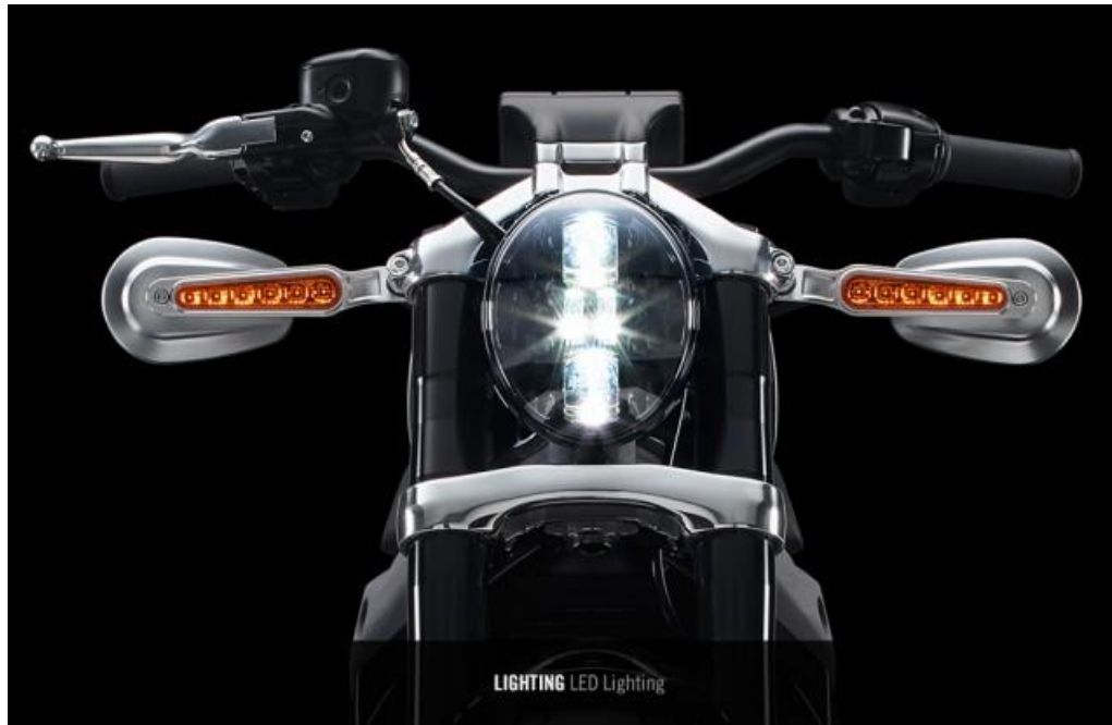
Image 30 – Front view of the Harley-Davidson Livewire electric prototype bike. As you can see there is no clutch lever as there is no clutch. An electric bike also has no gearbox so you cannot stall it. Power is available instantaneously just by twisting the throttle.
