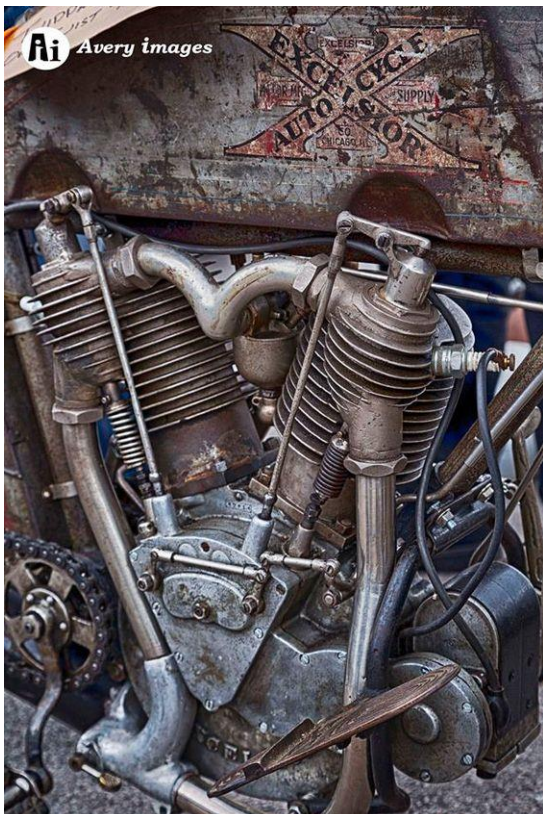
Image 4 - An early V-Twin engine of the Excelsior.
