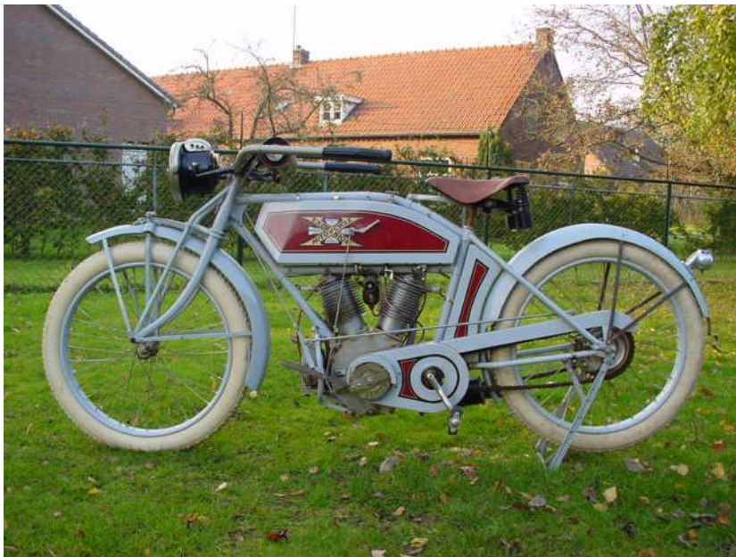
Image 6 - Pictured, a 1914 Excelsior. In 1910, Excelsior introduced an engine configuration they would become famous for, and one they would produce until 1929: the notable ‘X’ series. The first was the “Big X”, a V-Twin measuring 61 cubic inches (1,000 cc), which was the mainstay of Excelsior production through the 1910’s and into the 1920’s. This bike was originally single speed only, then with 2-speed and then 3-speed gearboxes.
