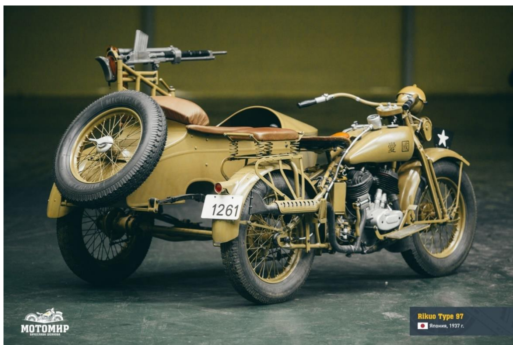
Image 44 - A military version Rikuo dubbed Type 97. These were made entirely from Japanese-made components.
