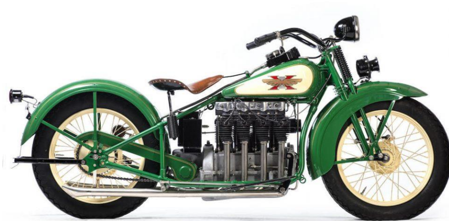
Image 22 - In 1928 the final version of the new Henderson Streamline series was introduced known as the Deluxe. The improvements included the addition of a front brake, rounded teardrop tanks and lower riding positions giving a thoroughly modernized appearance.
