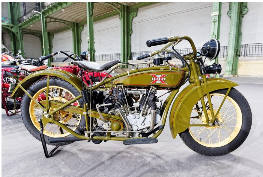
Image 8 - The Excelsior Super X was manufactured from 1925 to 1931. It was the most famous Excelsior motorcycle manufactured and was the first American forty-five cubic inch motorcycle (750 cc). Arthur "Connie" Constantine, Assistant Chief Engineer at the Harley-Davidson Motor Company, drew up plans for a mid-sized V-Twin to compete against the
