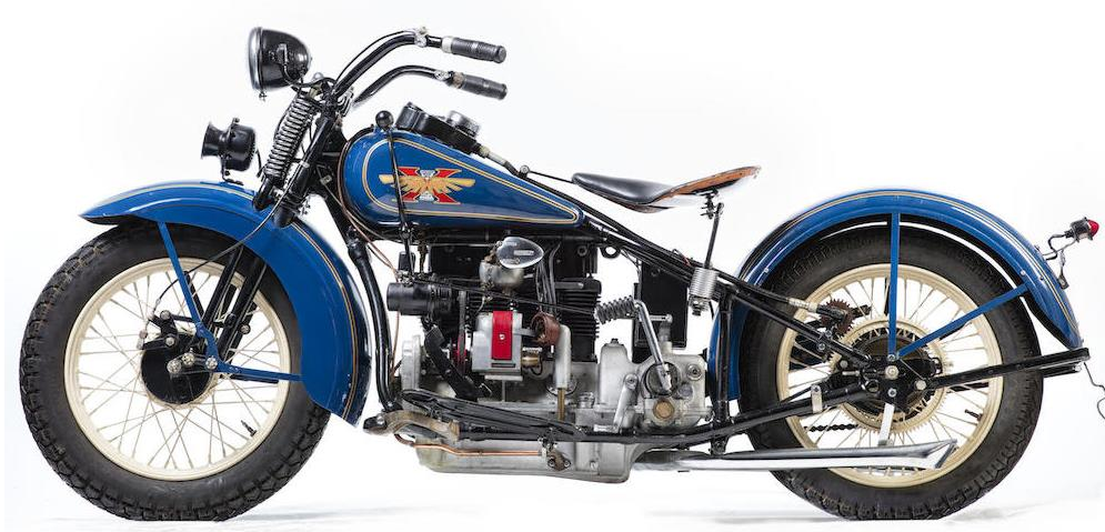
Image 24 - A final year production 1931 Excelsior – Henderson KJ Streamline model. It had a top speed in excess of 110 mph.
