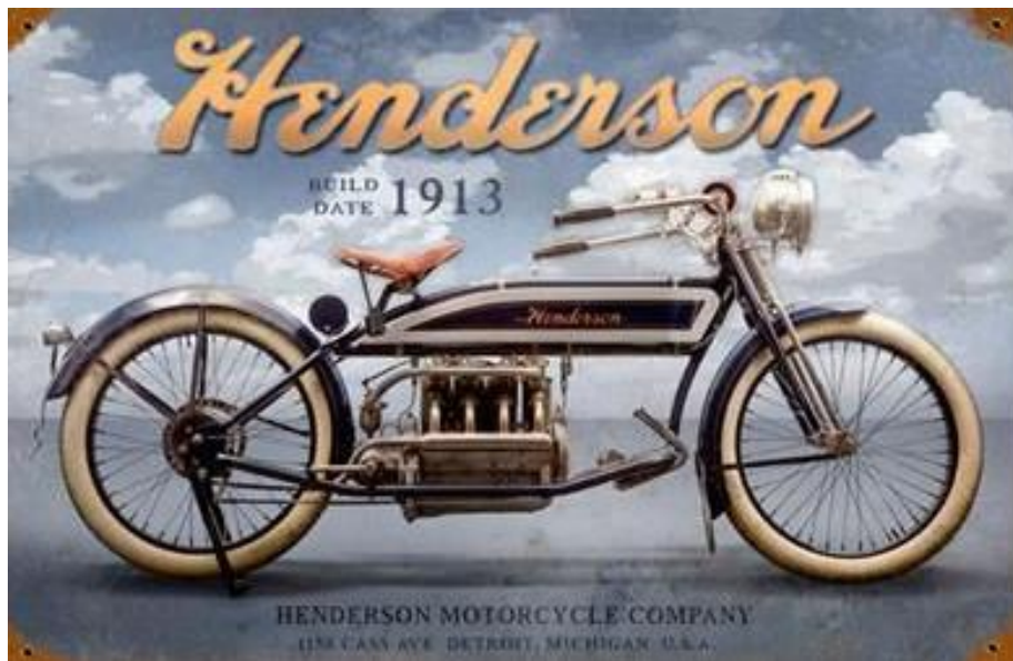
Image 11 - Henderson fours were the largest and fastest motorcycles of their time. Their ultra-long wheelbase also made them comfortable and stable at speed. Their in-line four-cylinder engine and long wheelbase would become Henderson trademarks.
