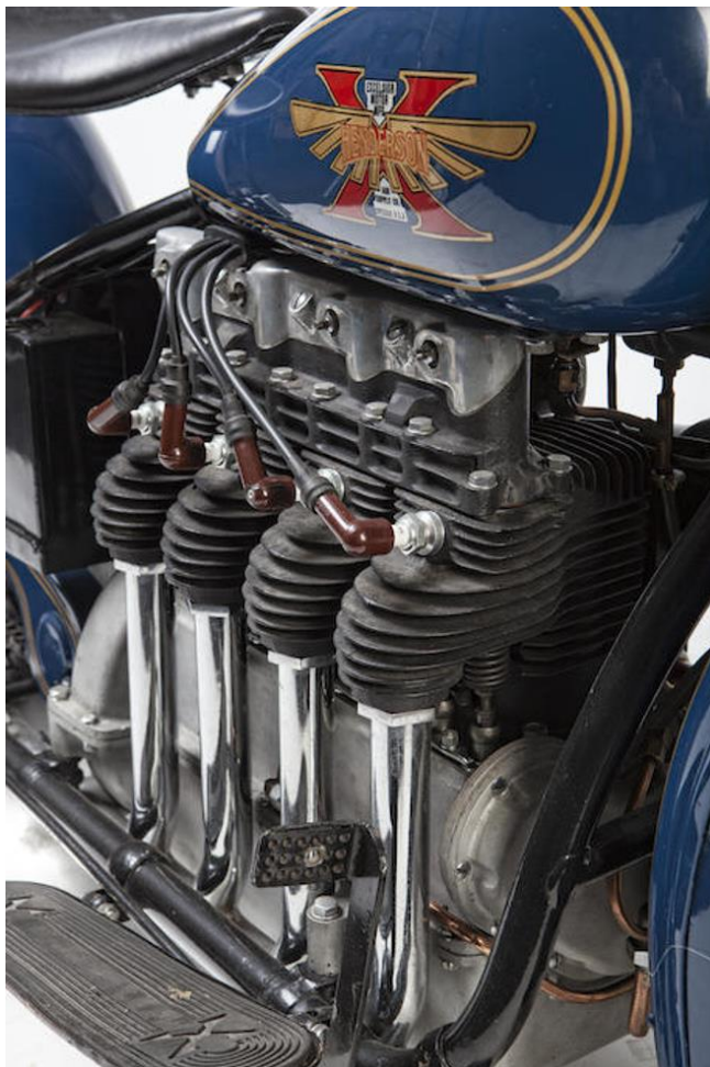
Image 25 - The Henderson 4-cylinder engine was globally acclaimed as a superb design. Indian also made a 4-cylinder motorcycle but not Harley-Davidson.
