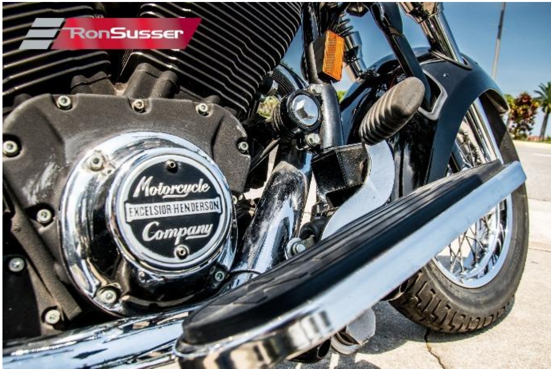
Image 37 - The 1999 Super X has a sophisticated DOHC 4-valve fuel injected V-Twin motor of 1386cc displacement with belt final drive.
