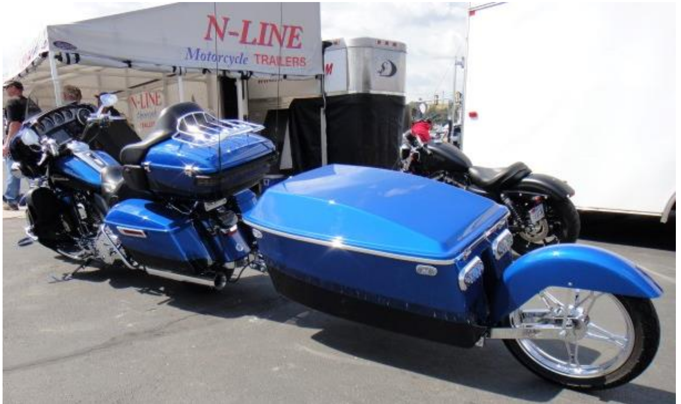
Sturgis Image 22 – Spotted this display on Lazelle Street in Sturgis, a motorcycle trailer that leans with the bike. N-Line Trailers specialize in single wheel motorcycle trailers which allow the bike and trailer to become one machine that leans into a curve. They also offer customization to meet your particular requirements. The trailer shown here is custom painted to match the hauling motorcycle.
